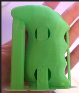
▲ Before removing support material from a test print
