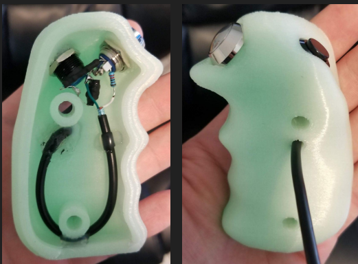
◀ The final right side handle with buttons installed
